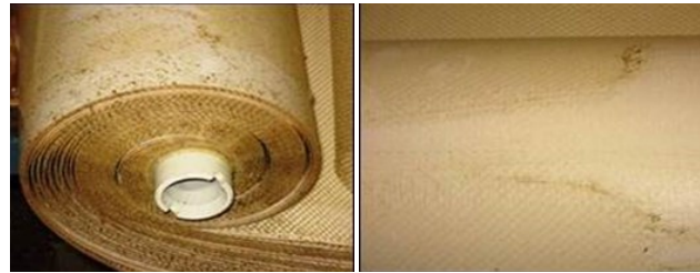
Figure 12. Disassembled SWRO membrane showing biofilm matrix
