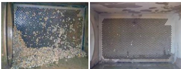
Figure 10. The effectiveness of the non-oxidizing biocide additive
